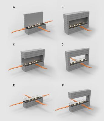
Decoflame recommends installing one or more glass shields in order to protect the mist from draught, while keeping it vivid.
