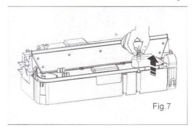
5. There are two clips, one on the left and one on the right hand side of the sump, holding down the sump. On the left side press in the clip with one hand and with the other lift the nozzle out of the clip. Repeat this for the right side (Fig. 8).
