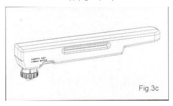
Fill the water tank with mains water. Distilled water must **not** be used.
